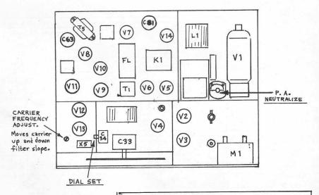
FIG. 2 - TOP VIEW, TUBE LOCATIONS
