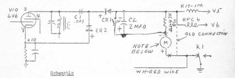
Components: Cl - .001 mfd., 1.000 wv, paper or ceramic type capacitor C2 - 2 mfd., 50wv or more, electrolytic (or paper) Rl - 47K ohm 1/2 watt resistor.
