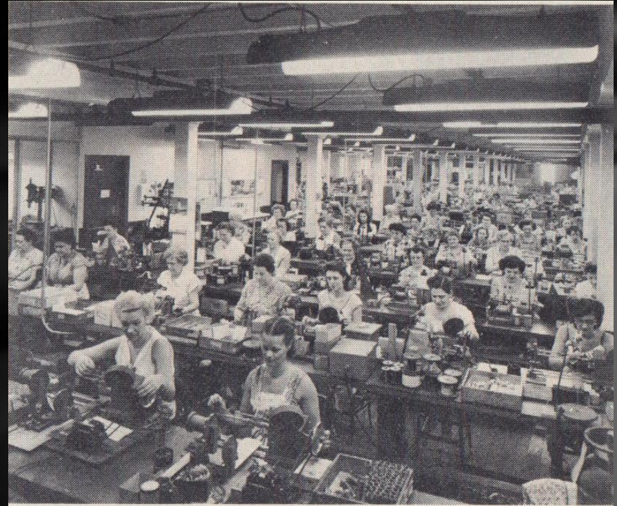
Coil-Winding Department has facilities for winding coils and chokes to any set of specifications in quantity.
