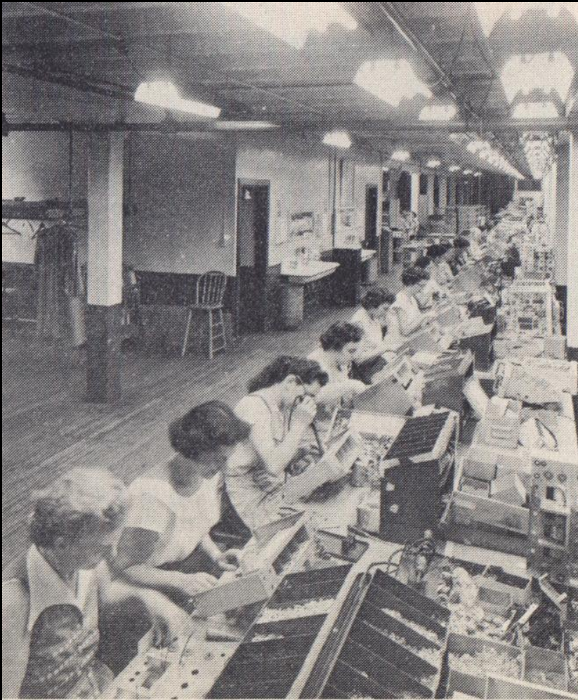
Assembly Line on HRO receiver chassis. Progressive steps install harness wiring, solder hundreds of connections.
