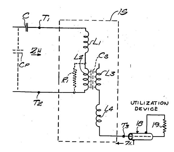
L1, L2 and Cp comprise a parallel resonant circuit...high impedance.
